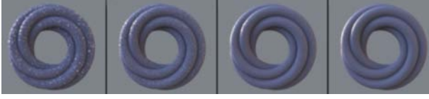
Figure 8: A low number of facets in the [JHY*14] model gives a glittery appearance (left), whereas with an increasing number of microfacets it tends to the classic smooth microfacets appearance (right). ©2014 Association for Computing Machinery, Inc. Reprinted by permission.
